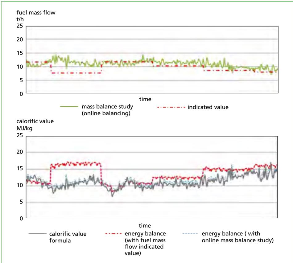
Figure 4: Fuel mass flow and calorific value over period of time
