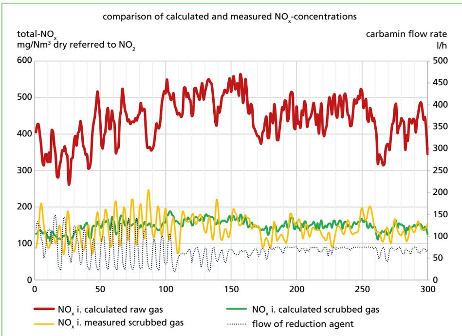
Figure 11: Calculated and measured total NO<sub>x</sub>-concentrations
