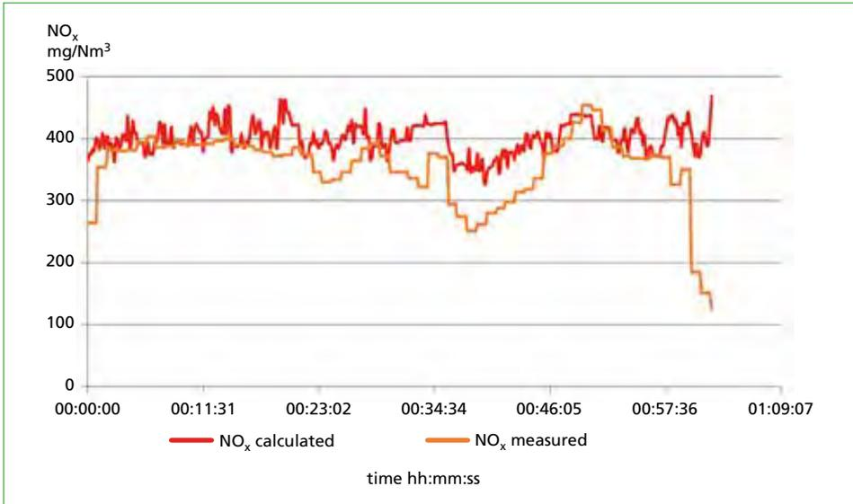
Figure 3:  $\text{NO}_x$ -raw gas value, measured and calculated by means of Opti-Link
