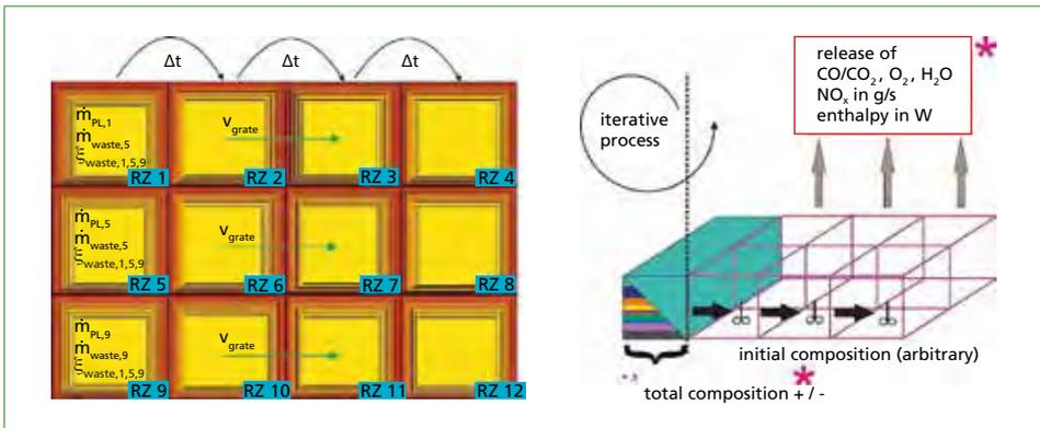
Figure 5: Schematic of the grate model (left); grate model consisting of a defined number of backward reactors (continuous stirred tank reactor elements)(right)
