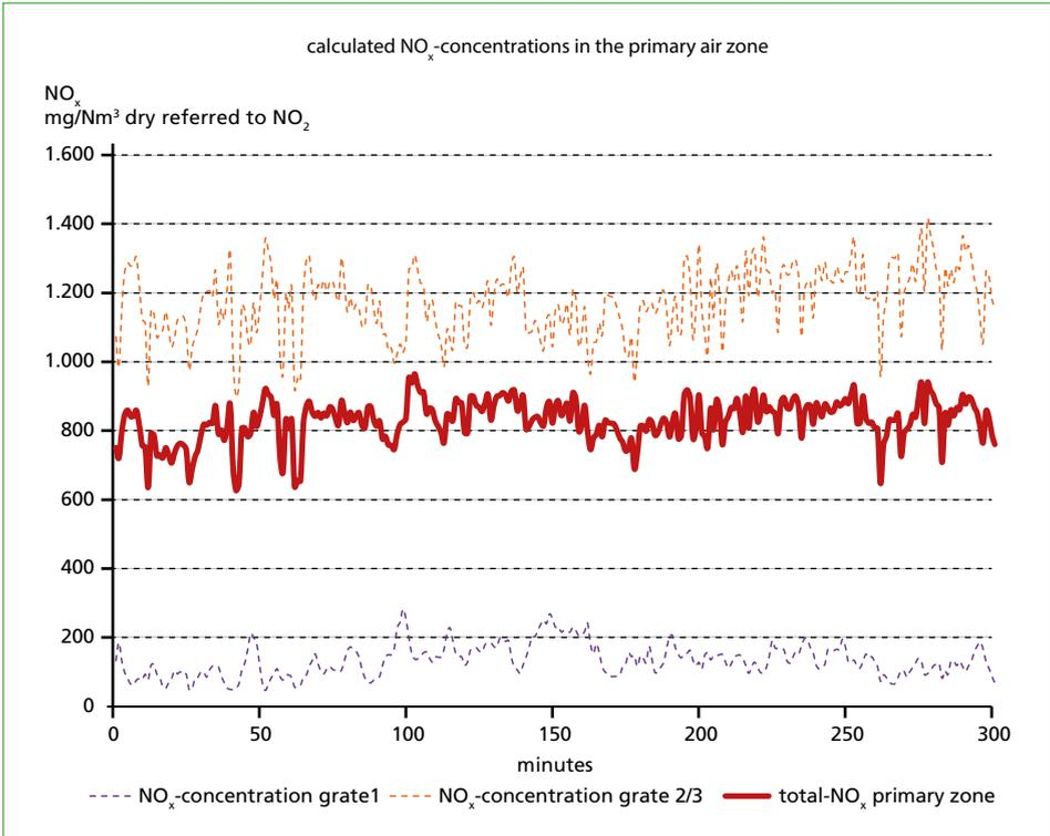
Figure 9: Calculated NO<sub>x</sub>-concentrations for different grate zones downstream the primary combustion zone
