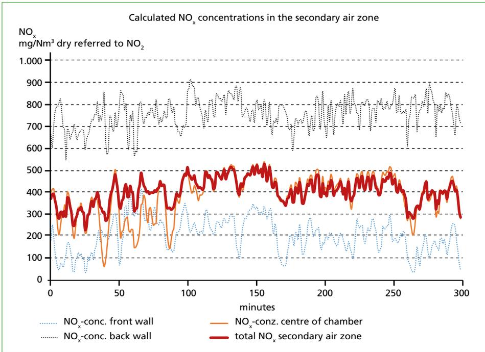
Figure 10: Calculated NO<sub>x</sub>-concentrations downstream the secondary air injection zone
