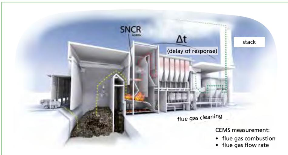
Figure 2: Delay time between SNCR and  $\text{NO}_x$  clean gas measured at the stack
