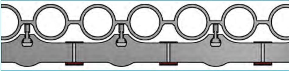
Figure 5: Horizontal cross section through SiC boiler tile system on the membrane wall
