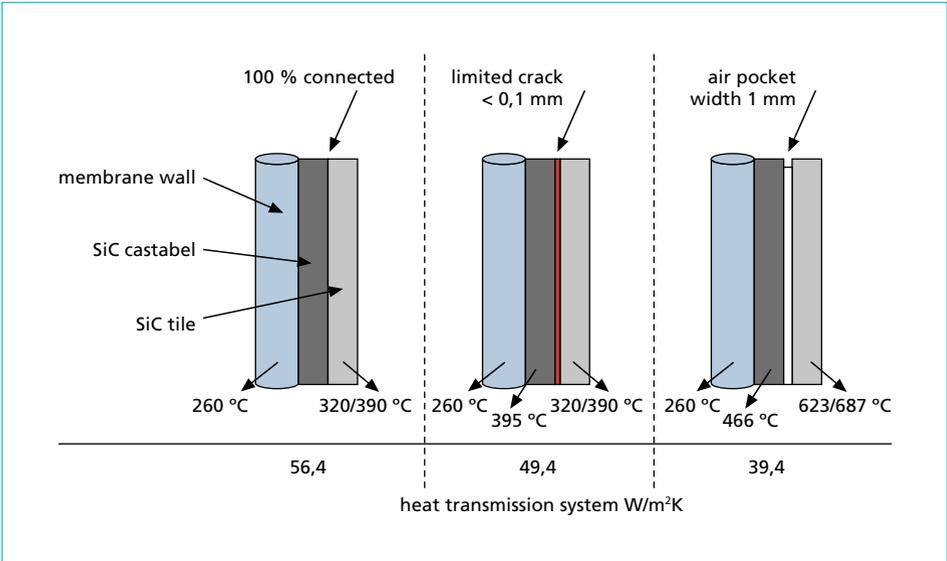
Figure 14: Effect of cracks between SiC tiles and castable
