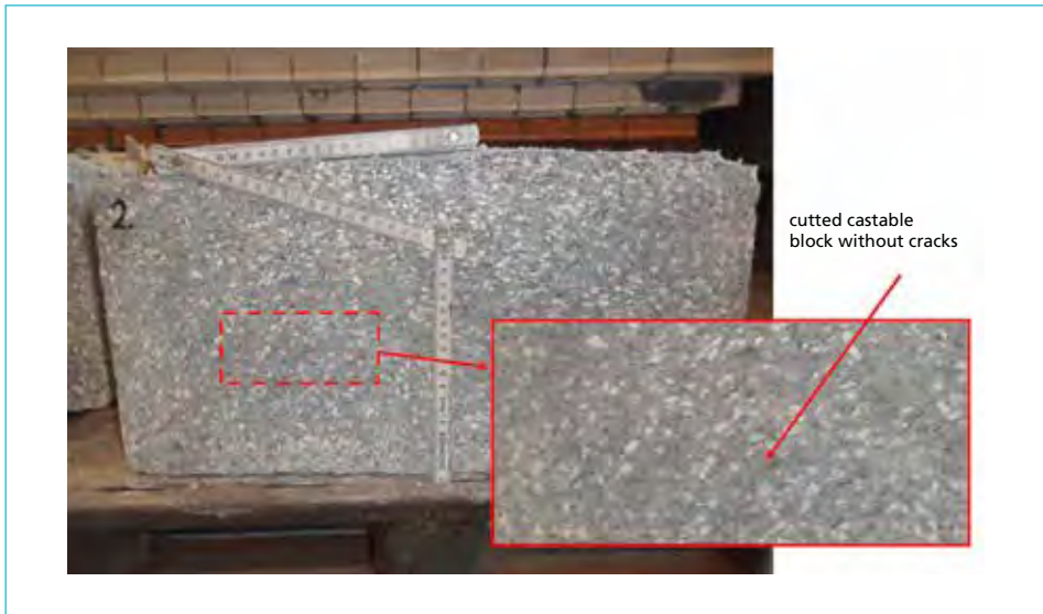
Figure 24: No cracking with High Performance Concrete HP100Q
