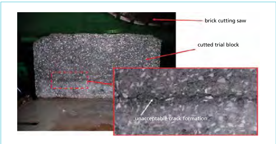
Figure 23: Unacceptable cracking of a conventional castable
