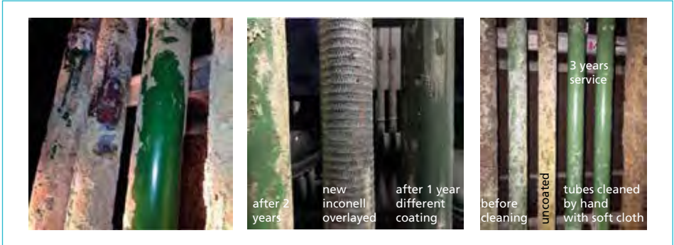
Figure 13: Tubes after one year and after three years before and after cleaning the ash by hand with a glove
