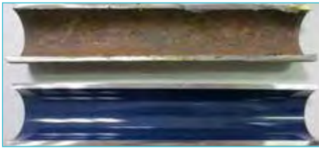
Figure 29: Coated/non coated elements from the condenser
