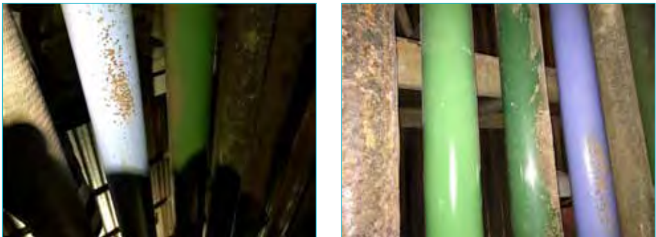
Figure 14: Tubes after four years with different ceramic quality after cleaning and some attacked tubes due to sand blasting last year without cover
