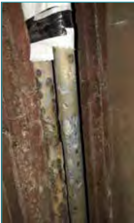
Figure 18: Tubes after one year with attack signs
