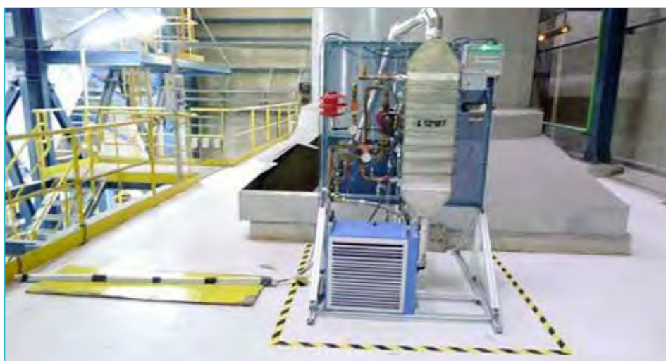
Figure 28: 5 kW fume condenser prototype at an urban waste power plant
