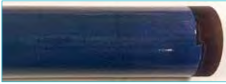
Figure 4: Water quenched from 850 °C to 20 °C (metal temperature)
