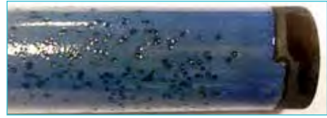
Figure 5: Softening defects appear at 900 °C (metal temperature)
