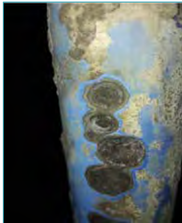
Figure 18: Tubes after one year with attack signs
