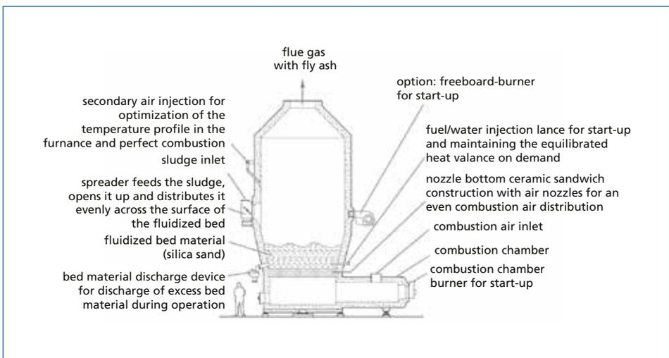
Figure 4: Basic principle of a fluidized bed incinerator
