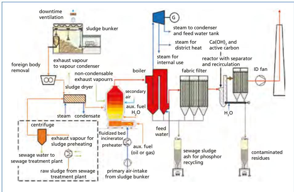
Figure 3: Sketch of mono-combustion plant
