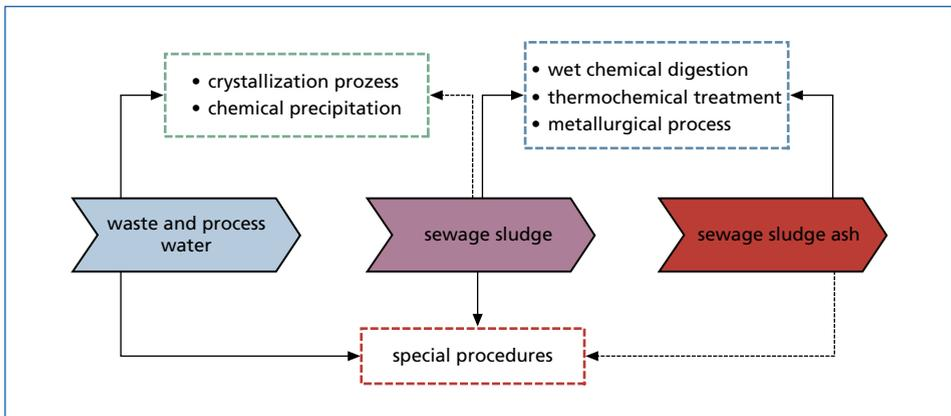
Figure 2: General overview of process approaches to recover phosphorus
