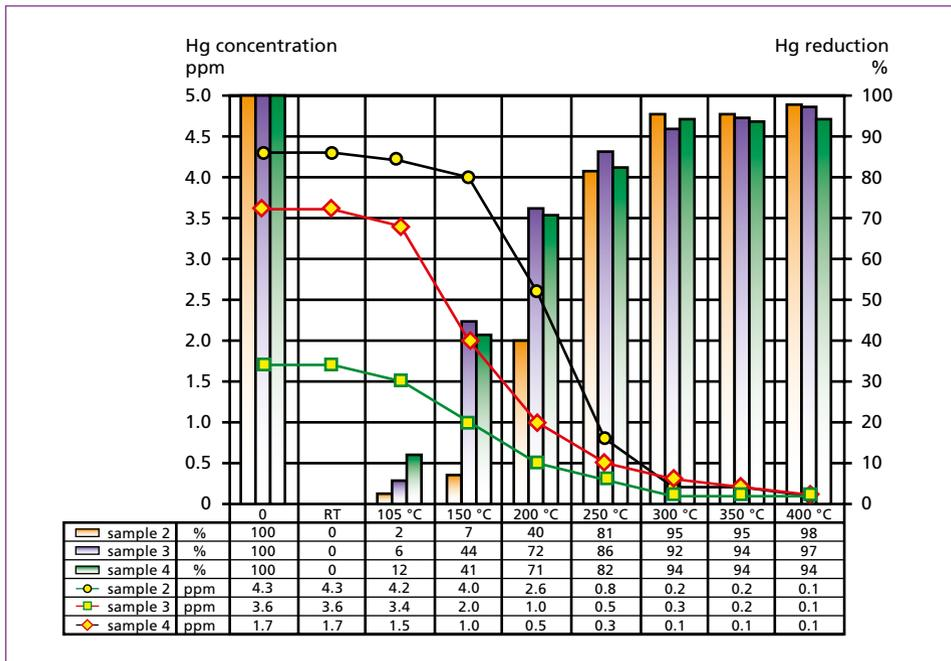
Figure 3: Results of the Hg evaporation tests carried out in the laboratory
