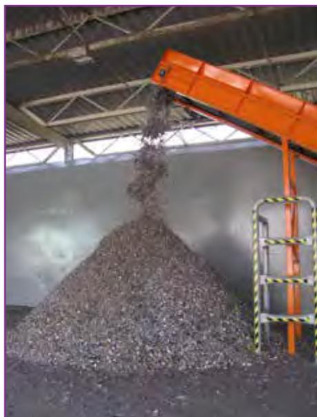
Figure 4: Refuse derived fuel from municipal waste after crushing
