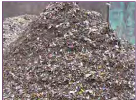
Figure 3: Subscreen fraction of the municipal waste
