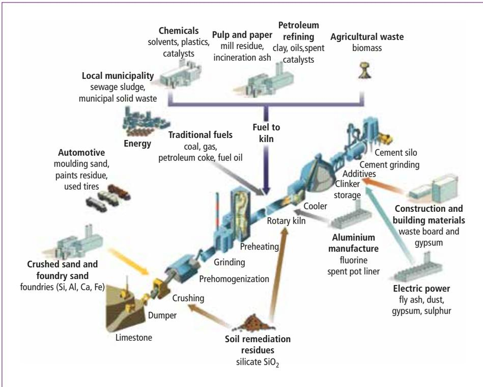
Figure 4: Examples of feeding alternative fuels and raw materials
