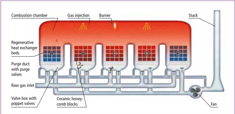
Figure 5: Components of the RTO
