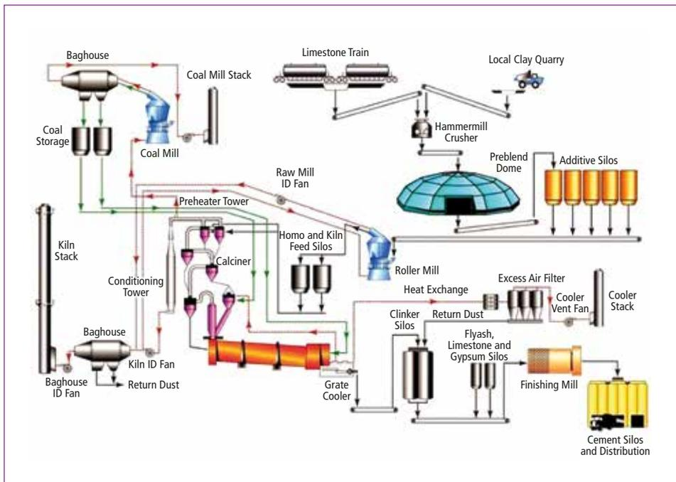
Figure 2: Cement plant flow chart
