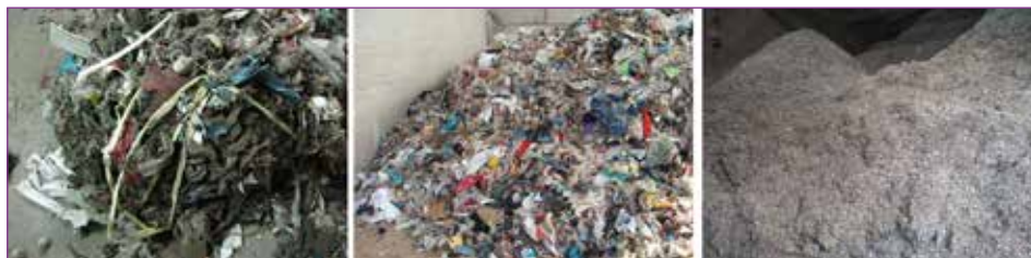
Figure 7: SRF low quality (left), SRF medium quality (centre) and SRF premium quality (right)
