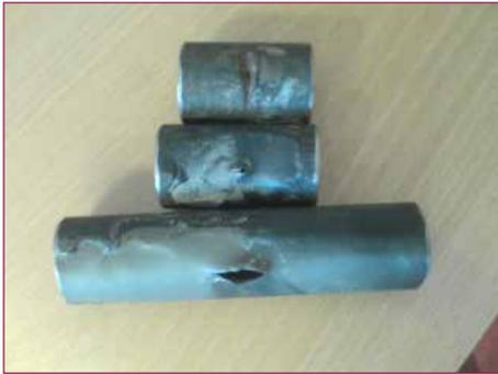
Figure 7: Water tubes with damages caused by steam soot blowing
