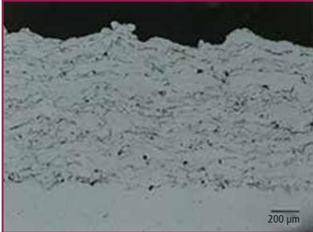
Figure 3: Micrograph of conventional *Twin Wire Arc Spray* (TWAS) process
