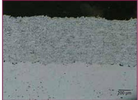
Figure 4: Micrograph of *High Velocity Arc Spray* (HVAS) process
