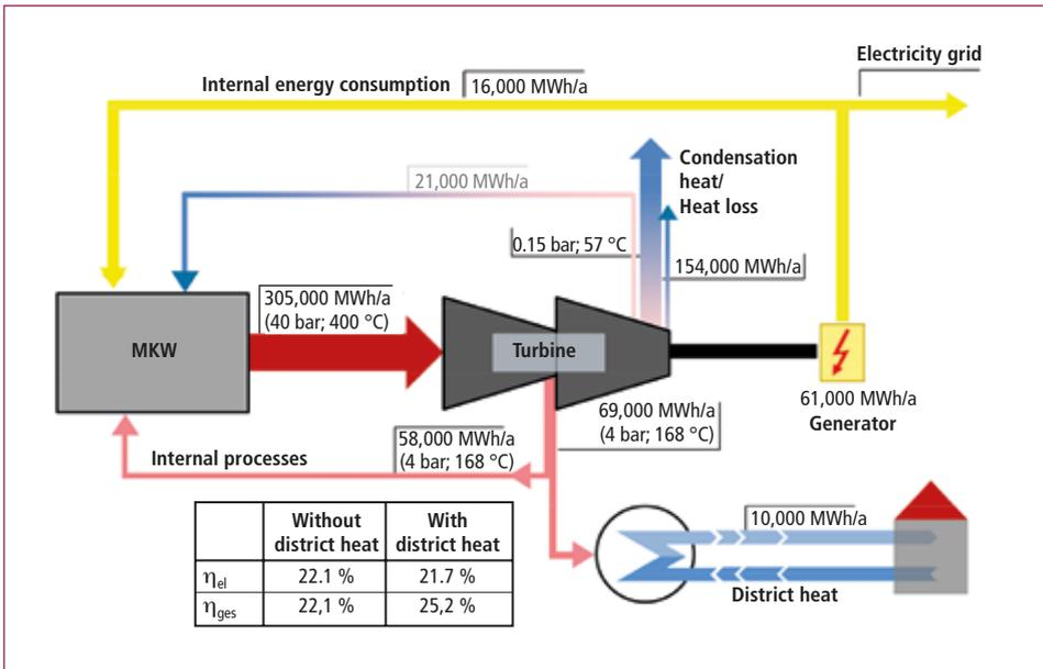
Figure 8: Simplified energy diagram for Weißenhorn MKW with heat coupling out
