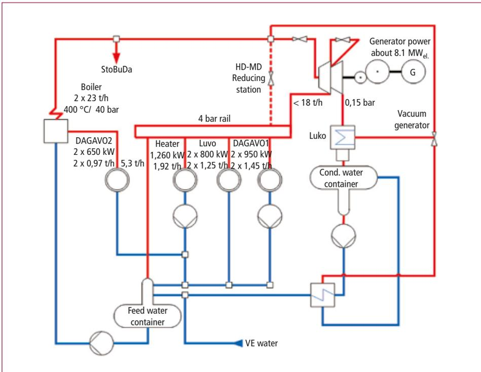
Figure 4: Block diagram of the water-steam system in Weißenhorn MKW, actual status
