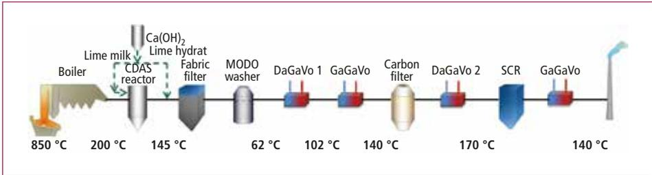
Figure 6: Flue gas route with temperatures in Weißenhorn MKW in the actual state
