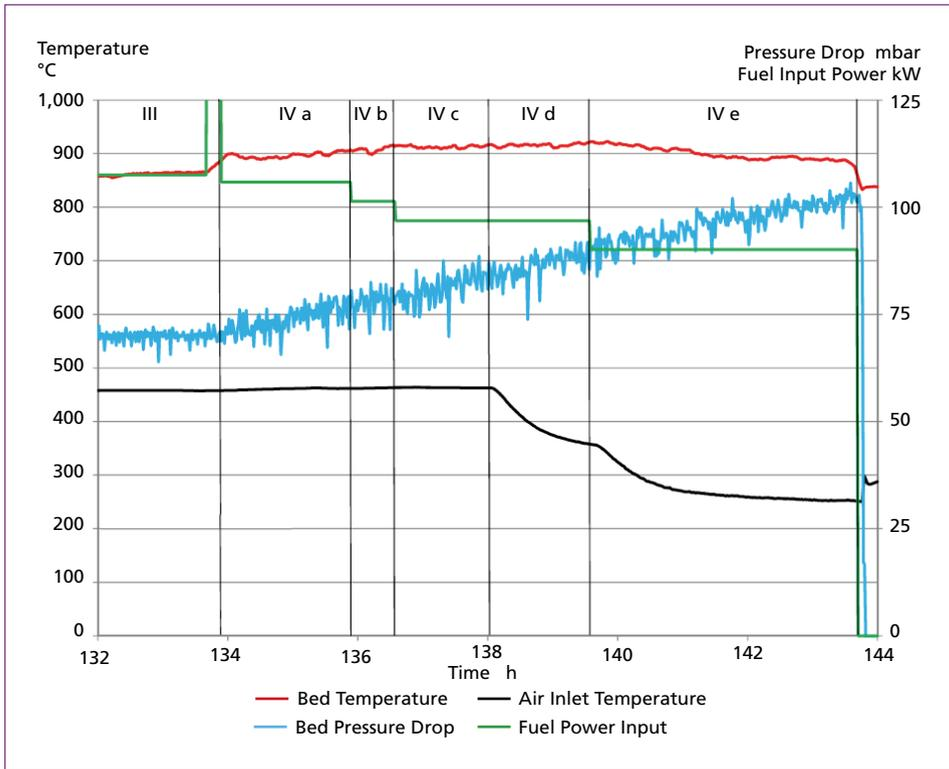
Figure 8: Development of characteristic parameters during combustion periods
