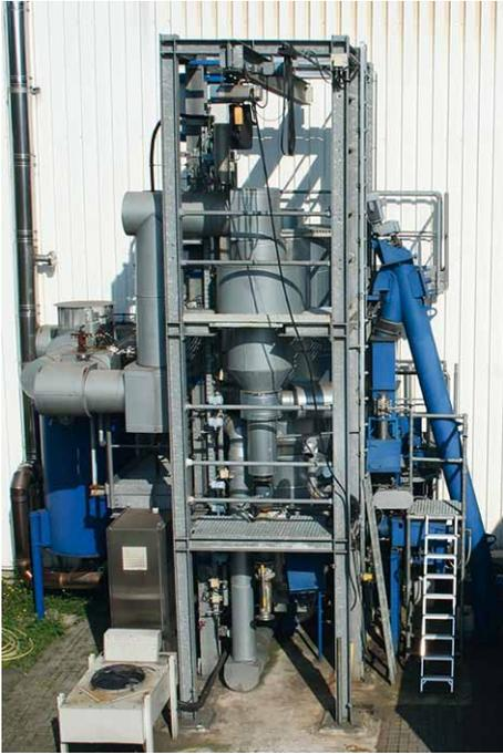
Figure 7: The 100 kW combustion unit at UMSICHT, Fraunhofer Institute
