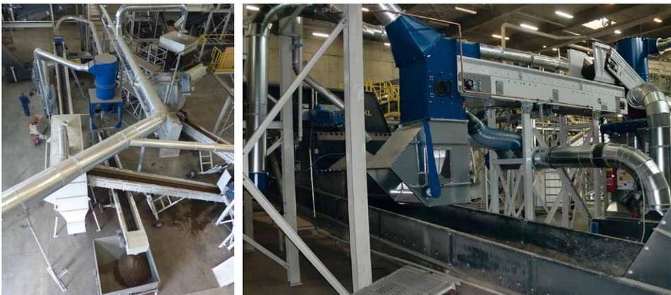
Figure 5: Photos showing the air sifter used in the MARSS plant
