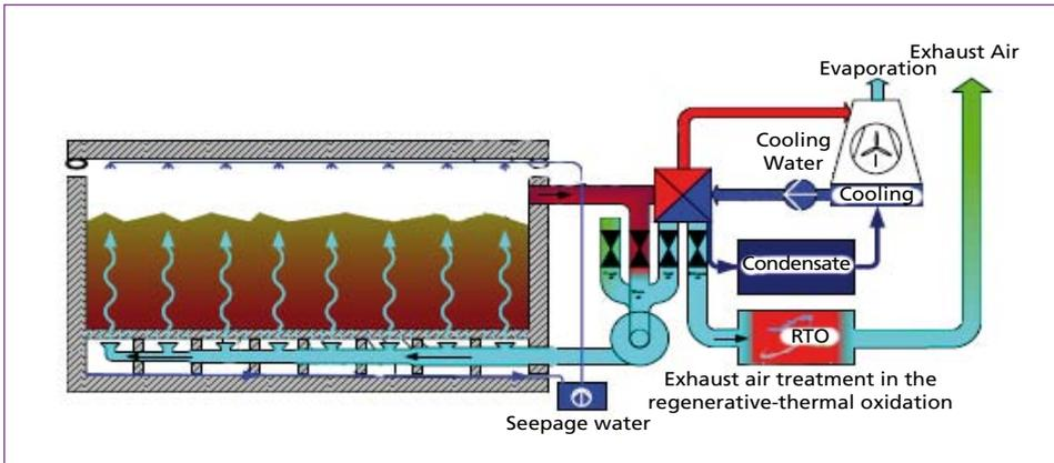
Figure 4: Impression of the rotting box system used in the RegEnt MBT plant
