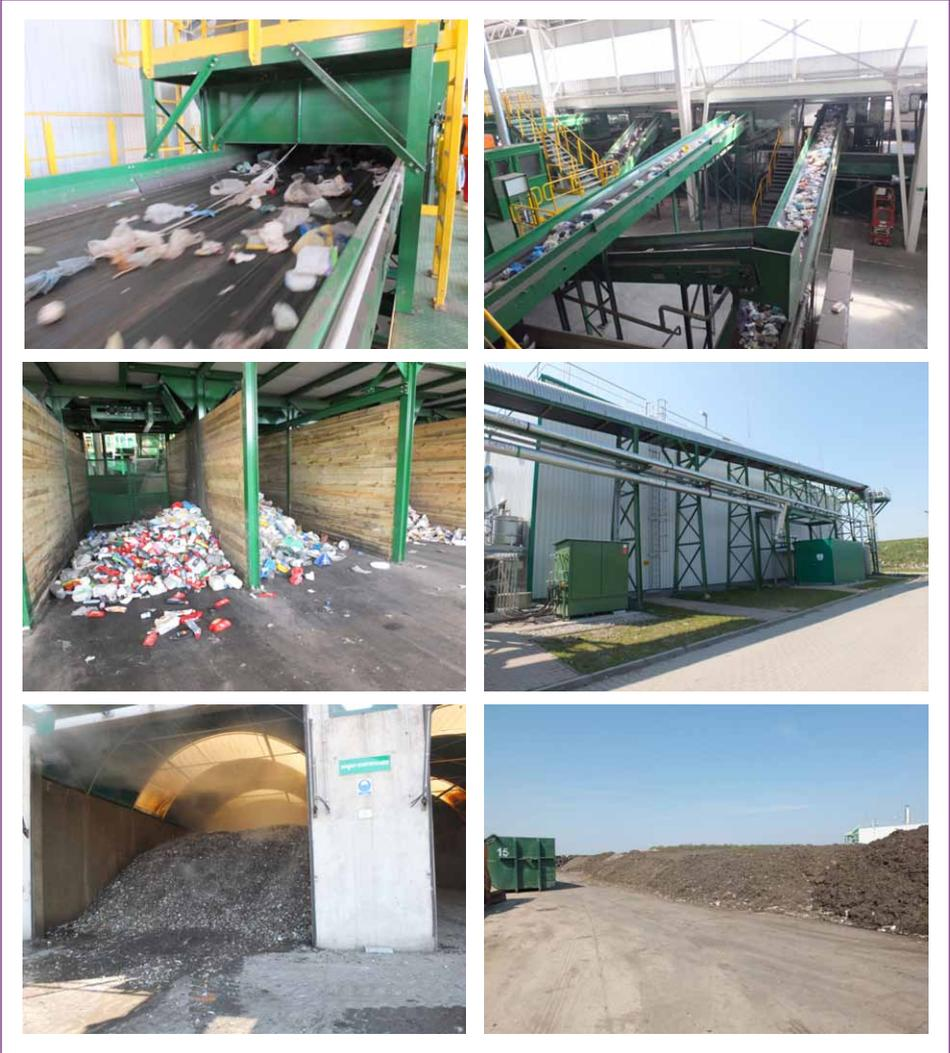
Figure 6: Advanced MBT plant, based on dry anaerobic digestion
