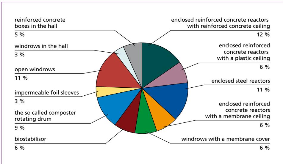
Figure 4: Dominating aerobic stabilization technologies used in Polish MBT plants
