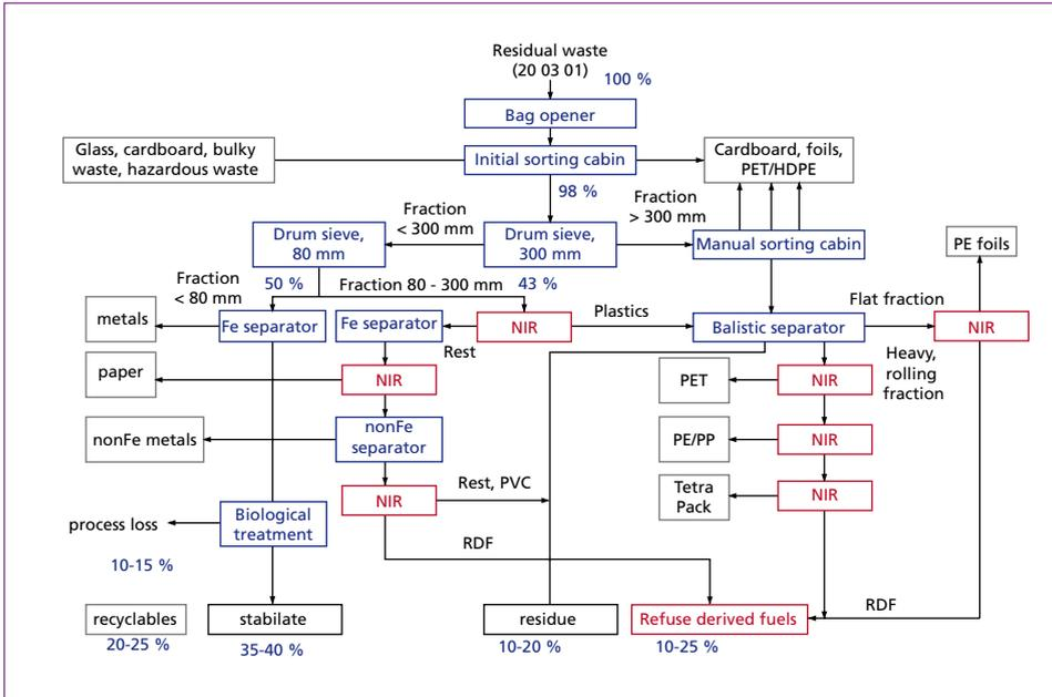
Figure 5: The concept of MBT technology, with mass balance used in some of Polish MBT plants
