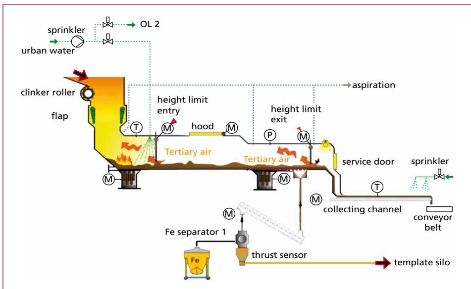
Figure 5: Dry bottom ash discharge scheme
