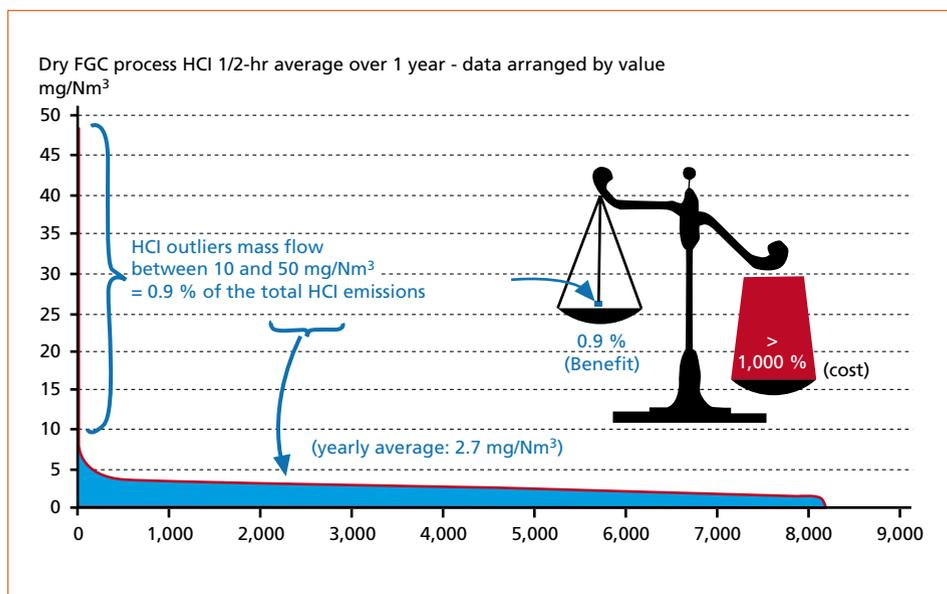
Figure 3: Same data as in Figure 2 but arranged by value; on this example, lowering the ½-hr HCl ELV from 60 to 10 mg/Nm<sup>3</sup> would reduce the already very low HCl emitted flow by 0.9 % but would require over 1,000 times more reagent in mass
