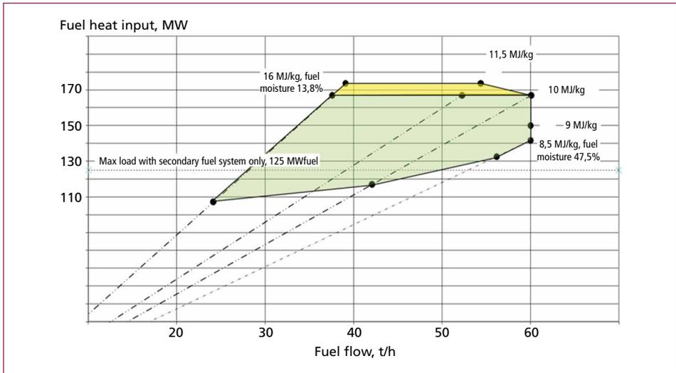
Figure 4: Combustion diagram of the plant
