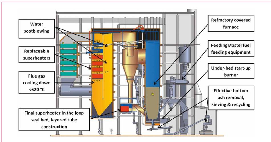
Figure 2: Special features of SRF concept
