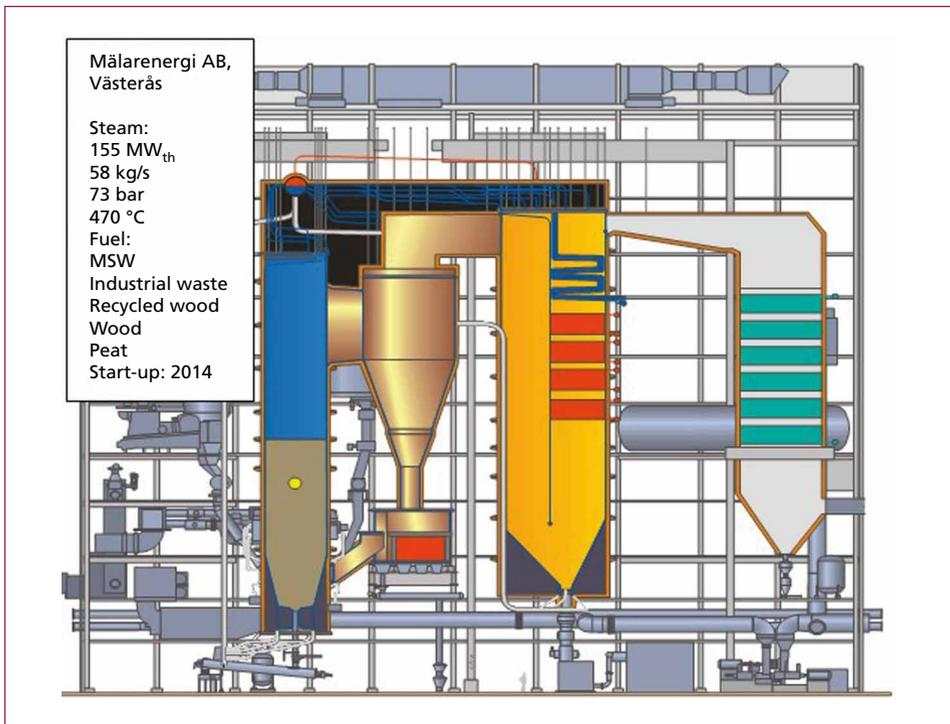
Figure 3: Sideview of world's largest recovered fuel fired boiler, Mälarenergi Unit 6
