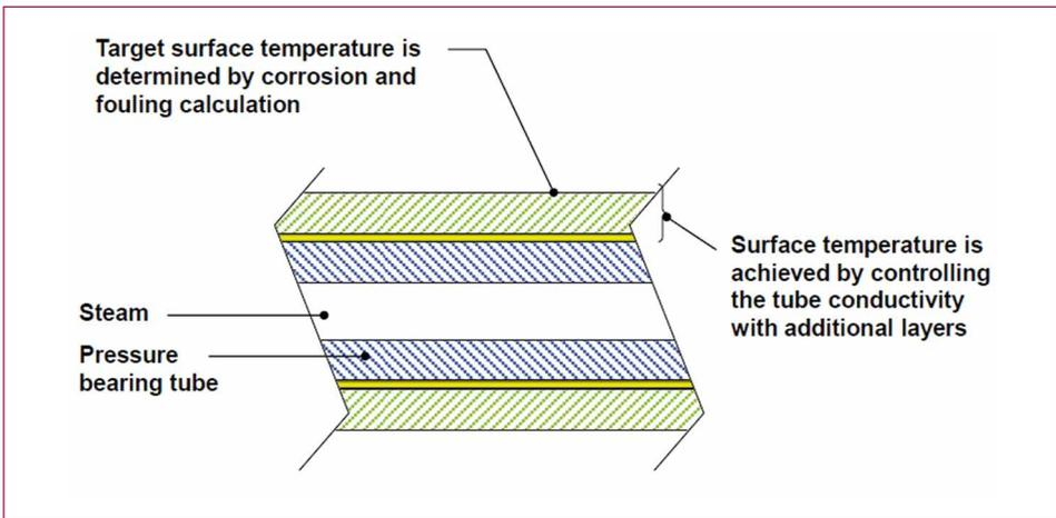
Figure 1: Multi layered tube construction of fluidized bed heat exchanger
