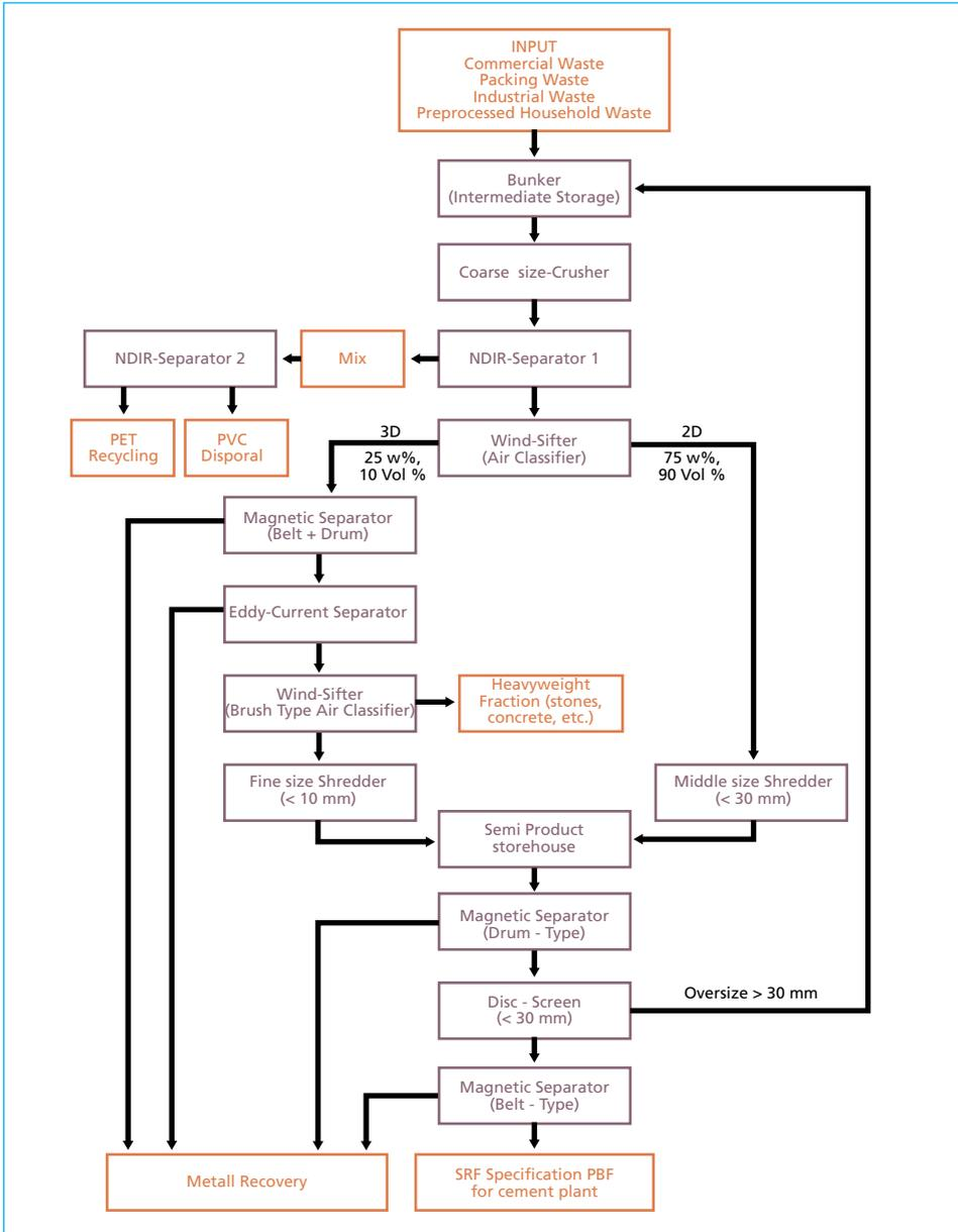
Figure 6: Simplified flow scheme of the SRF production plant Thermo Team
