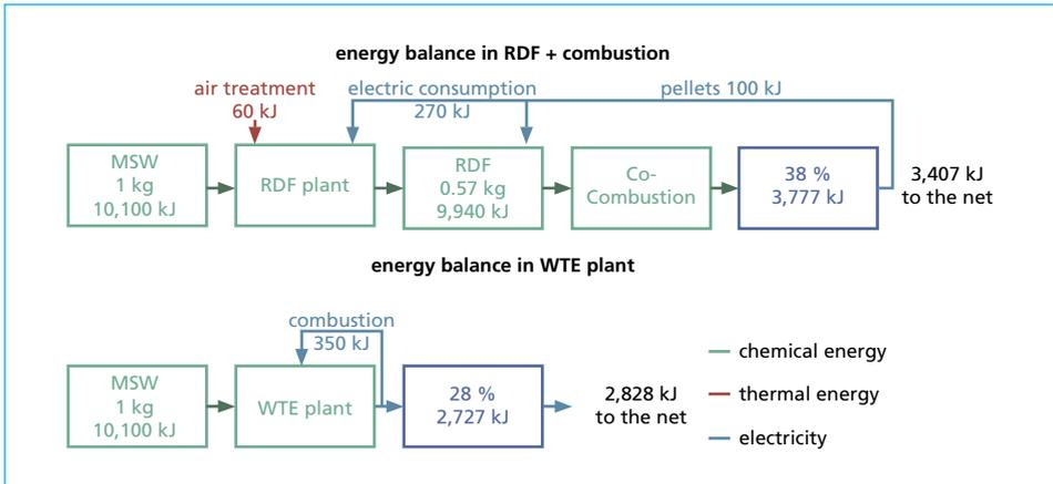
Figure 2: Comparison of the energy balance in case of use of MSW directly in WTE plant or in the case of the supply chain in Fusina
