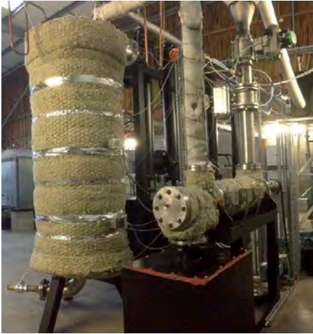
Figure 3: Pilot plant with BAF reactor
