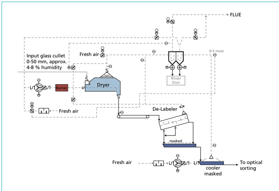
Figure 1: Flowchart of dry cleaning *sublimation* of waste glass fraction
