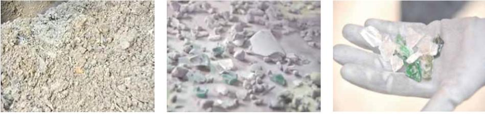
Figure 7: Cleaning effect of glass fractions from WIP slag
