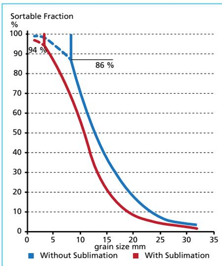
Figure 8: Increase in the range of sortable grain size
