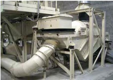
Figure 4: Cooling and de-dusting vibratory feeder
