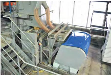
Figure 5: Sensor-based separator for glass fraction with feed system; installation in Bratislava
