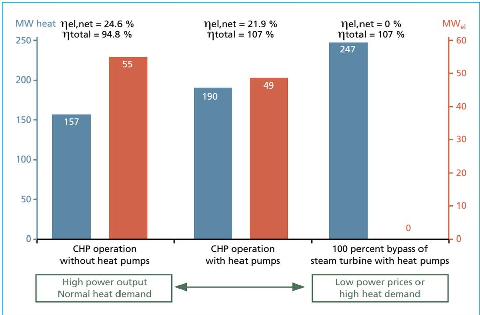
Figure 6: Modes of operation in relation to energy recovery at Copenhagen; assuming operation is at nominal conditions; outputs and efficiencies are net, i.e. after subtraction of parasitic consumption
