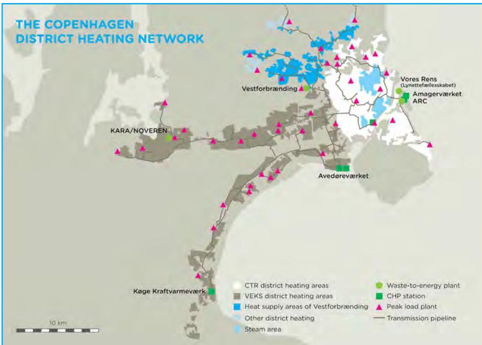
Figure 2: The Copenhagen district heating network, showing several WtE facilities as well as other CHP plants including peak load boilers
