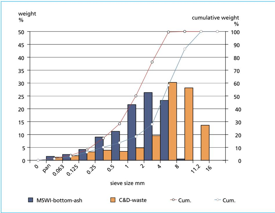
Figure 1: Size distribution of MSWI-bottom-ash and construction and demolition waste
