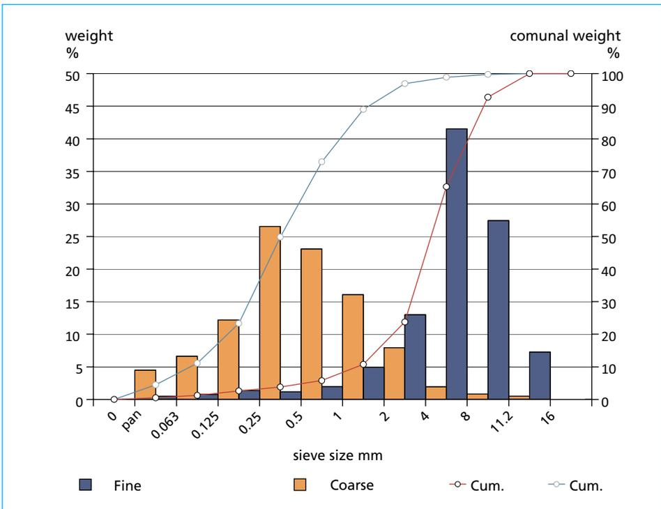
Figure 2: Particle size distribution of construction and demotion waste processed with the ADR technology
