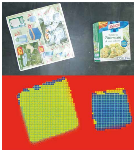
Figure 8: An advertising leaflet, and a board packaging of similar colours (above), and as seen with the thermal camera (below): yellow = paper, blue = board
