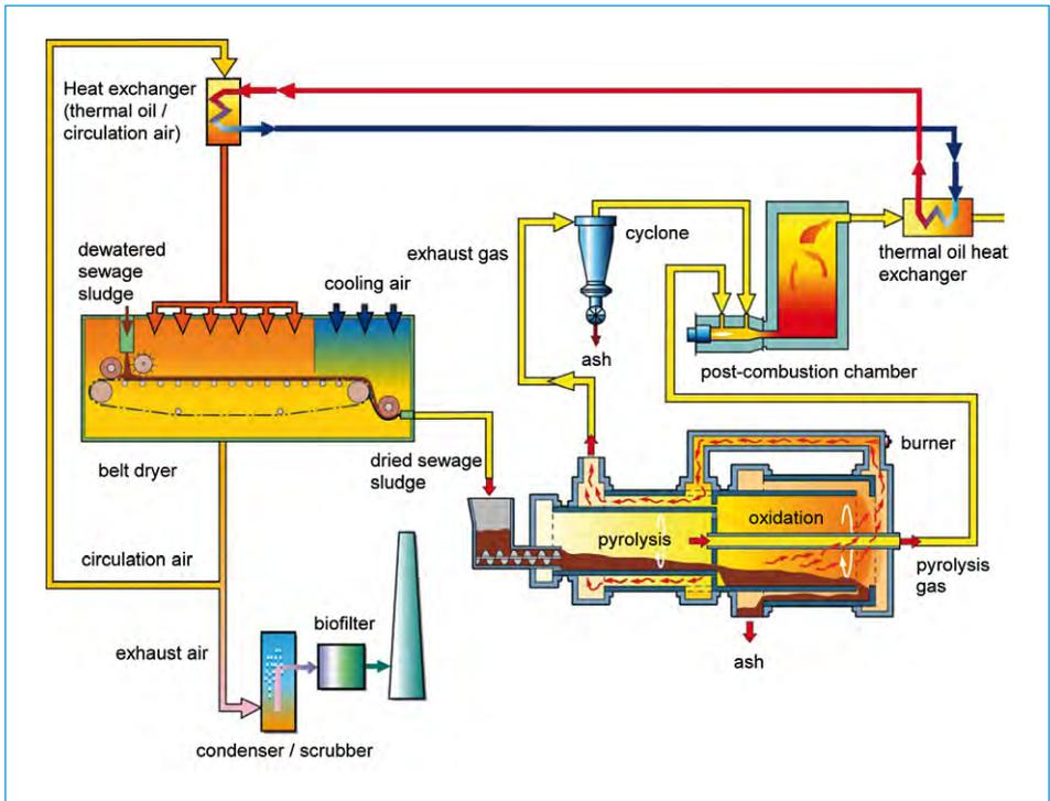
Figure 4: Simplified flow sheet of an existing Pyrobustor-facility in ARA Pustertal
