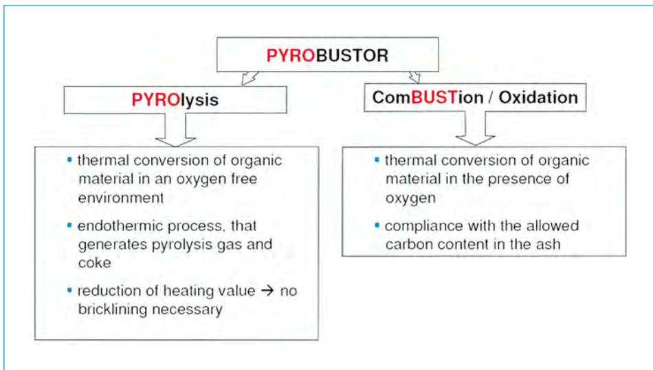
Figure 1: Explanation of the wording Pyrobustor
