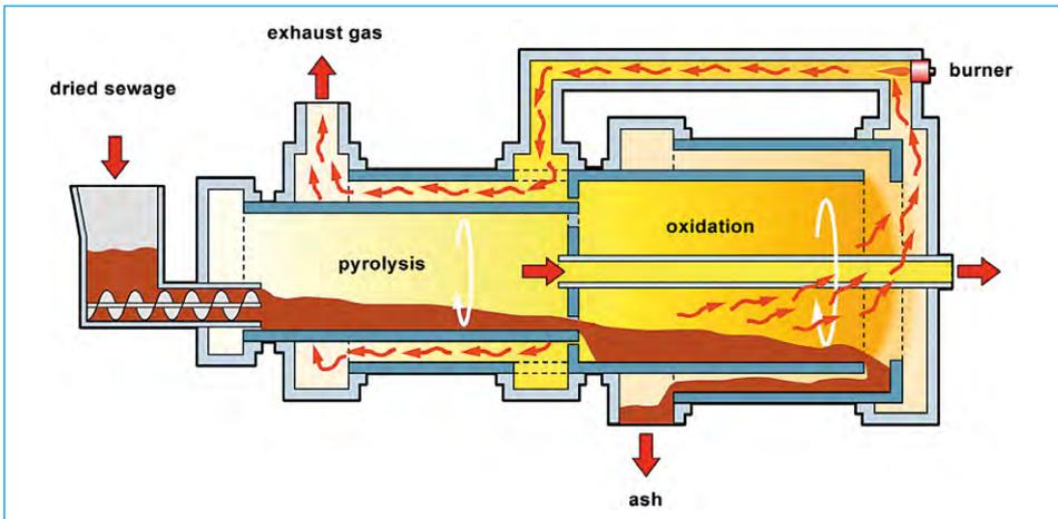
Figure 2: Schematic representation of the Pyrobustor incineration unit
