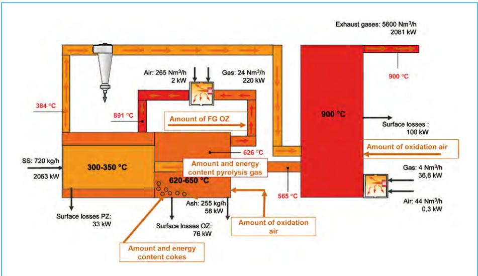
Figure 6: Summary of the unknown process parameters based on the recorded data of the plant in South Tyrol
