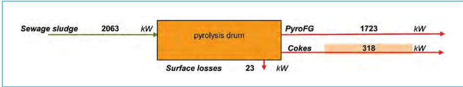
Figure 10: Energy balance pyrolysis zone
