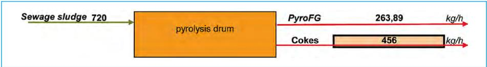
Figure 9: Mass balance pyrolysis zone
