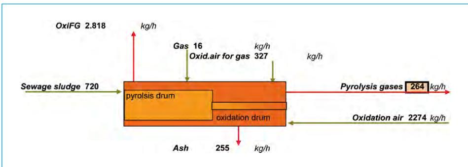
Figure 8: Mass balance Pyrobustor
