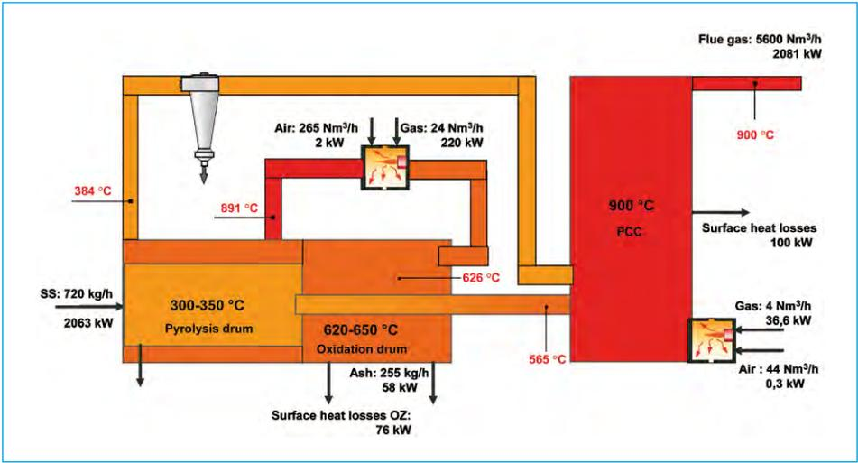
Figure 5: Summary of the known process parameters based on the recorded data of the plant in South Tyrol
