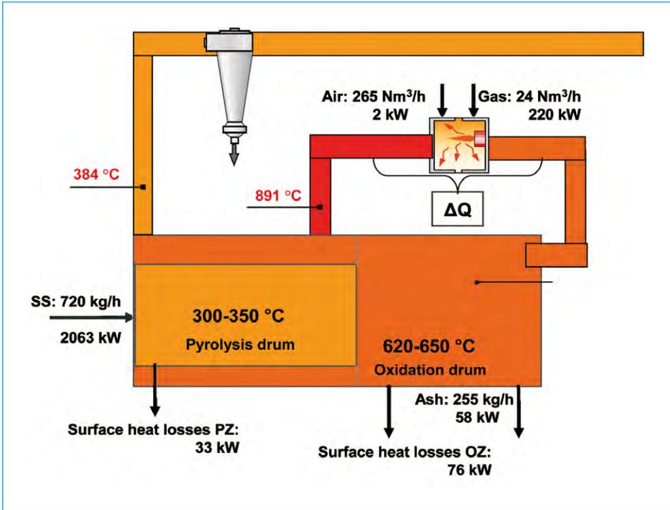
Figure 7: Determination of the exhaust gas amount ex oxidation zone
