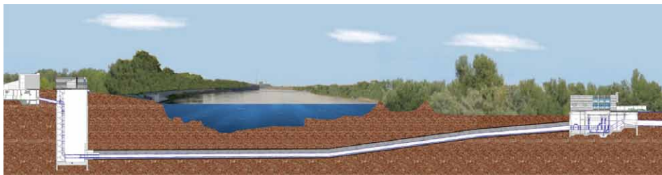
Figure 3: The Passage under the bed of Vistula River – visualization by MPWiK S.A. Extension and rehabilitation of the Wastewater Treatment Plant Czajka
