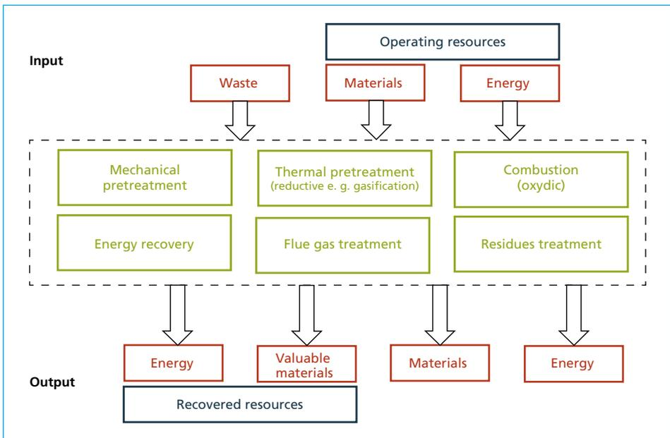
Figure 2: Overview of the unit operations and materials and energy streams within thermal waste treatment technologies
