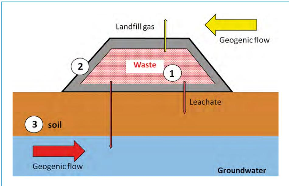
Figure 2: Concept of final storage landfill: substance flows of the landfill are insignificant in comparison to geogenic flows in the atmosphere, hydrosphere and pedosphere
