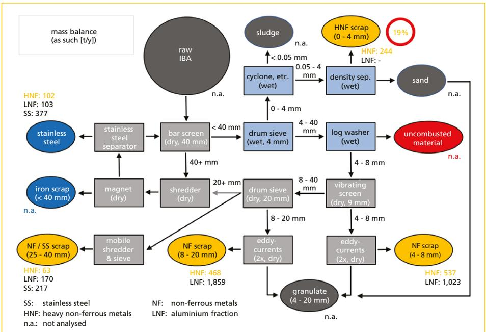
Figure 8: Overall mass balance pure light (LNF) and heavy (HNF) non-ferrous metals
