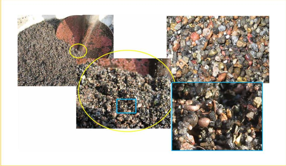
Figure 6: Impression of the heavy non-ferrous metals mixture obtained by density separation
