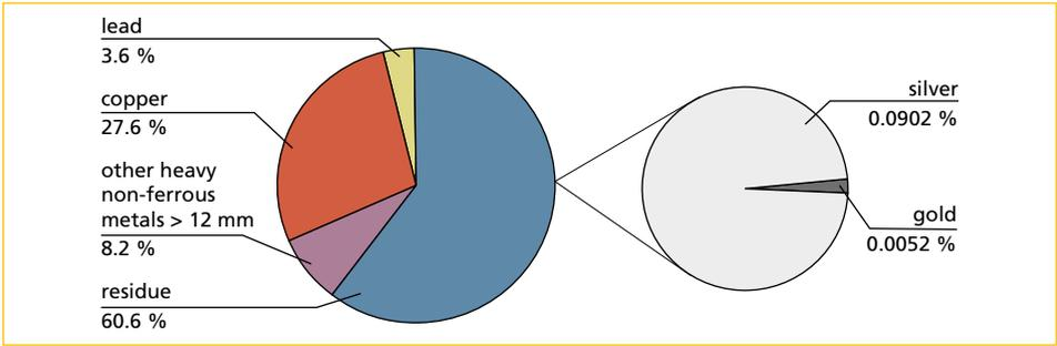
Figure 7: Composition of heavy non-ferrous metals (HNF) < 4 mm obtained from sand
