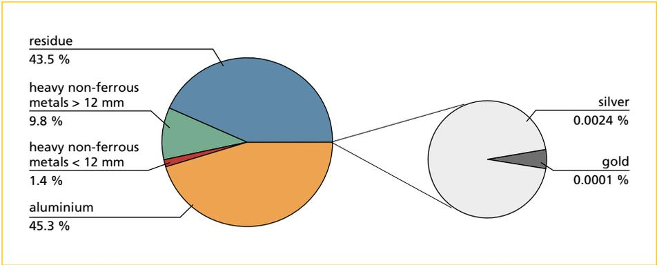
Figure 4: Composition of 8–20 mm non-ferrous mixture
