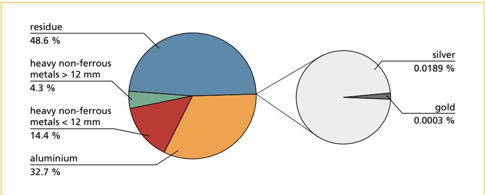
Figure 5: Composition of 4–8 mm non-ferrous mixture
