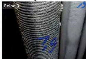
T_{RG}/T_{Of} = 680^{\circ}\text{C}/465^{\circ}\text{C} , flächige Abzehrung
