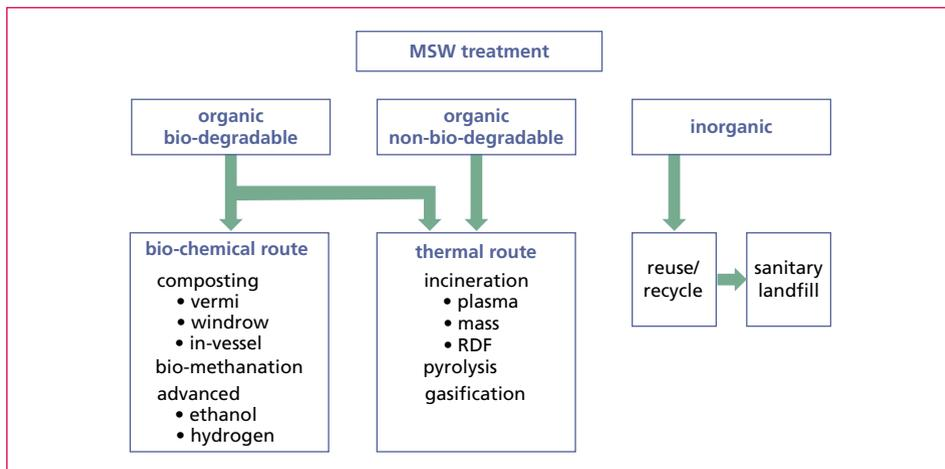
Figure 2: MSW processing technologies
